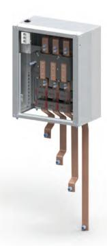
In the incoming module, an INP 1000-2000 switch disconnector or other manufacturer's switch disconnector (after consultation) or compact circuit breaker with rated current (630-1600 A) can be installed. The circuit breaker or switch disconnector can be equipped with a motor-drive mechanism. It is also possible to install ammeters, voltmeters or a network analyser.
