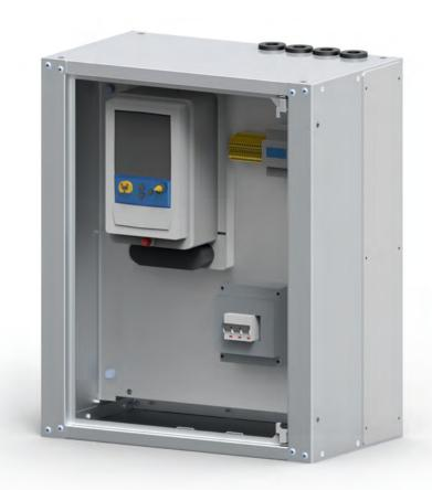
The metering module is used to install an energy meter for billing purposes, designed as a panel for installation of one to four meters. The metering system is also equipped with a metering terminal block, e.g. SKa, and voltage circuits protection.
